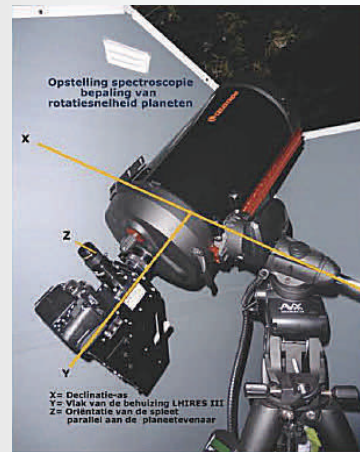
Fig. 3: Alignment of the spectrograph and camera, while capturing spectral recordings of planet Jupiter
